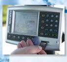
**DATA TRANSFER** For the easy transfer of data to a PC via memory card for record keeping or invoice preparation.
