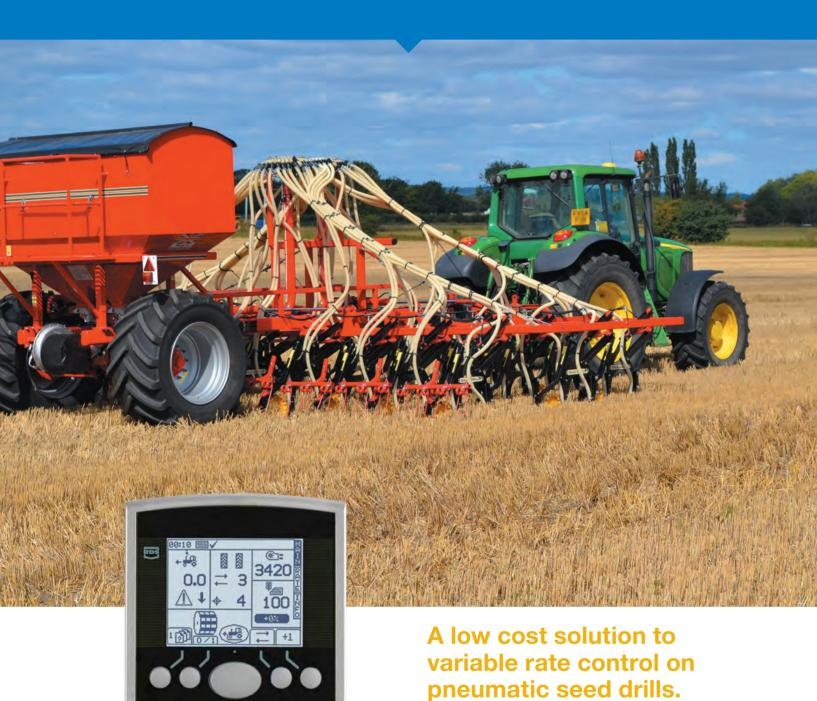
Using the experience gained from the Precision Farming enabled PSi Artemis (over 1000 in the field), the *Artemis Lite* is designed specifically for drills with a single pneumatic metering unit. Typically this would be a close-coupled 3-point linkage mounted drill.
