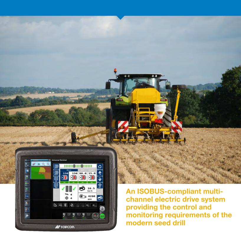
With increasing adoption of variable rate technology, the requirement for control of multiple products and now ISOBUS, the *Artemis* system has now been developed to work with compliant UT's.
