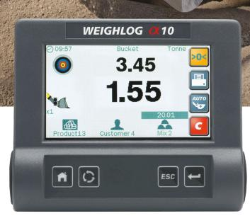
The RDS **WEIGHLOG**  $\alpha$ 10 incorporates the latest colour touchscreen technology providing a user-friendly on-board weighing system that can be used for trailer and hopper loading, batch blending or check weighing.
