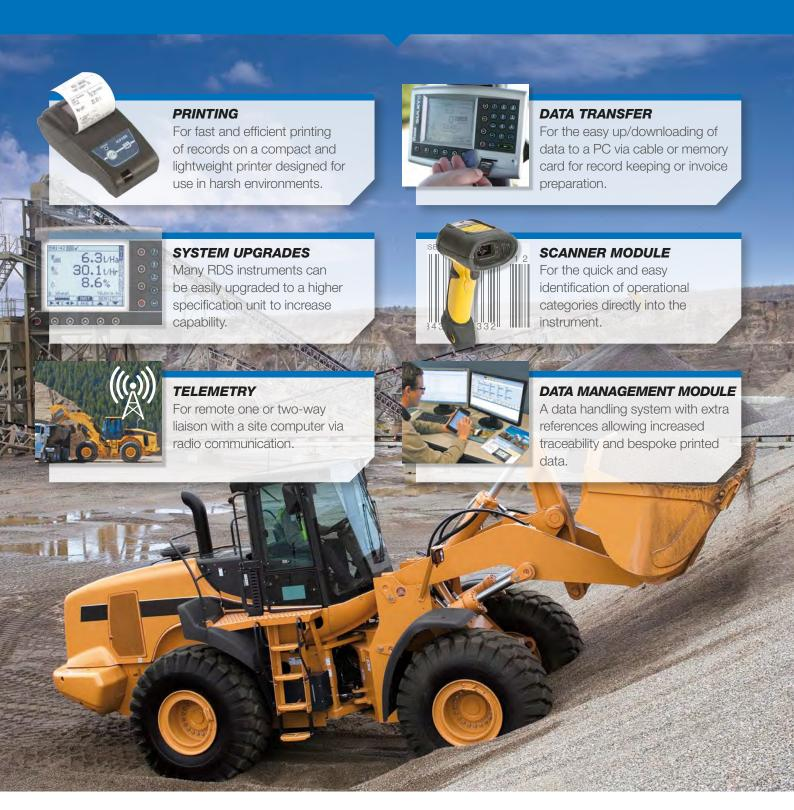
RDS offers a wide range of system extras to expand the functionality of your on-board weighing system
