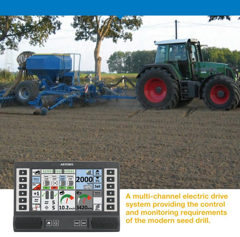
With increasing adoption of variable rate technology and requirement for control of multiple products on the modern seed drill, the **iSOCAN Artemis** is the ideal user-interface to provide intuitive operation.
