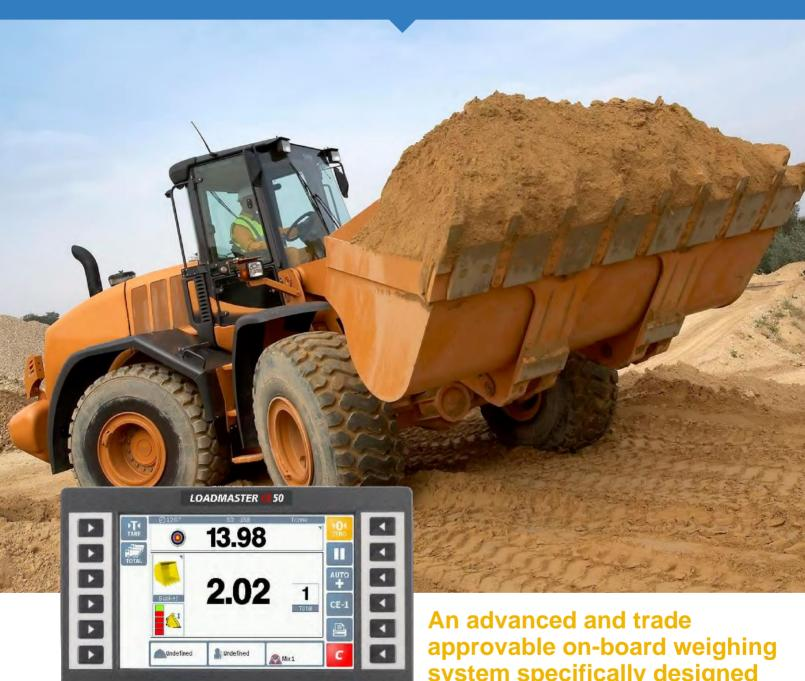
The RDS LOADMASTER 50 is a highly accurate, onboard weighing system for loaders that helps increase loading efficiency, cutting vehicle movements on site, increasing safety and ensuring trucks are correctly loaded first time.
