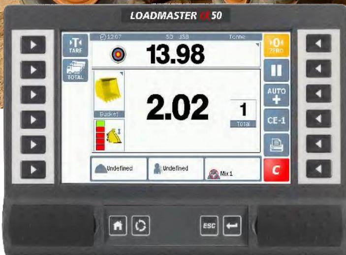
**An advanced and trade approvable on-board weighing system specifically designed for wheeled loaders operating in the toughest environments**
